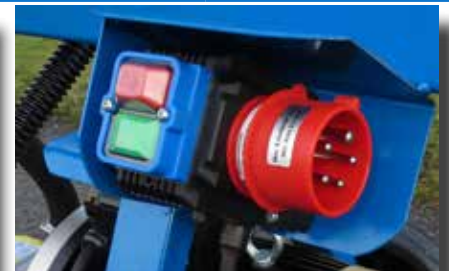
Motor protection with phaseinverter 3-phase 400 V
