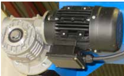
Wormgear equipped electric motor in the upper part
