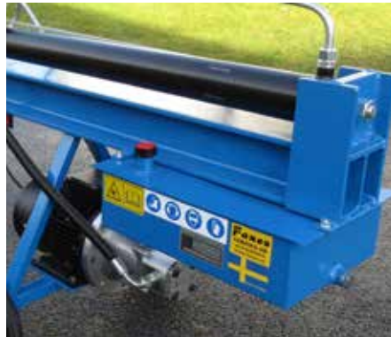
Separat oiltank at the rear ELH1100
